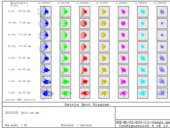
(a) Central wavelength of 360nm at  $m = 62$  in the blue channel
