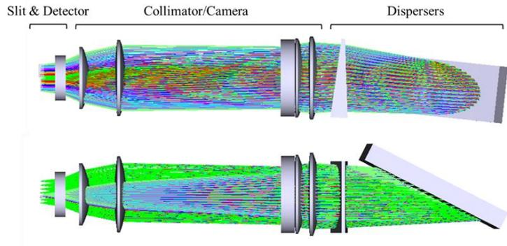
Figure 11. Double-pass optical design for the channel-spectrographs
