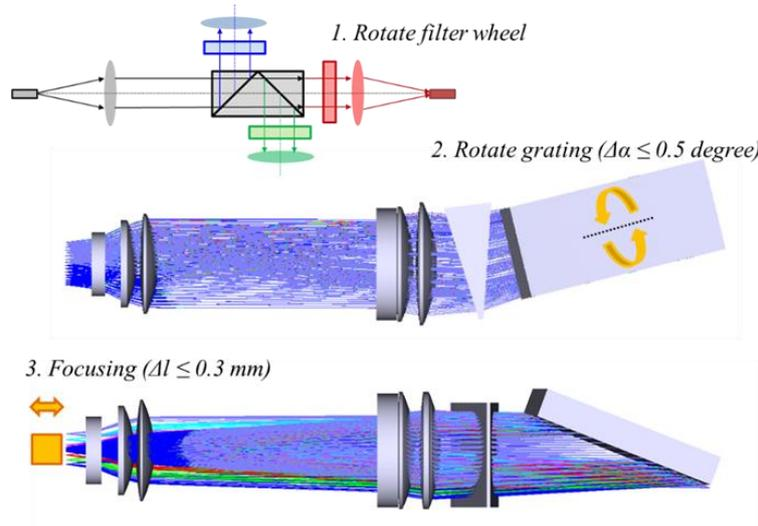
Figure 6. Operation scheme for switching working windows
