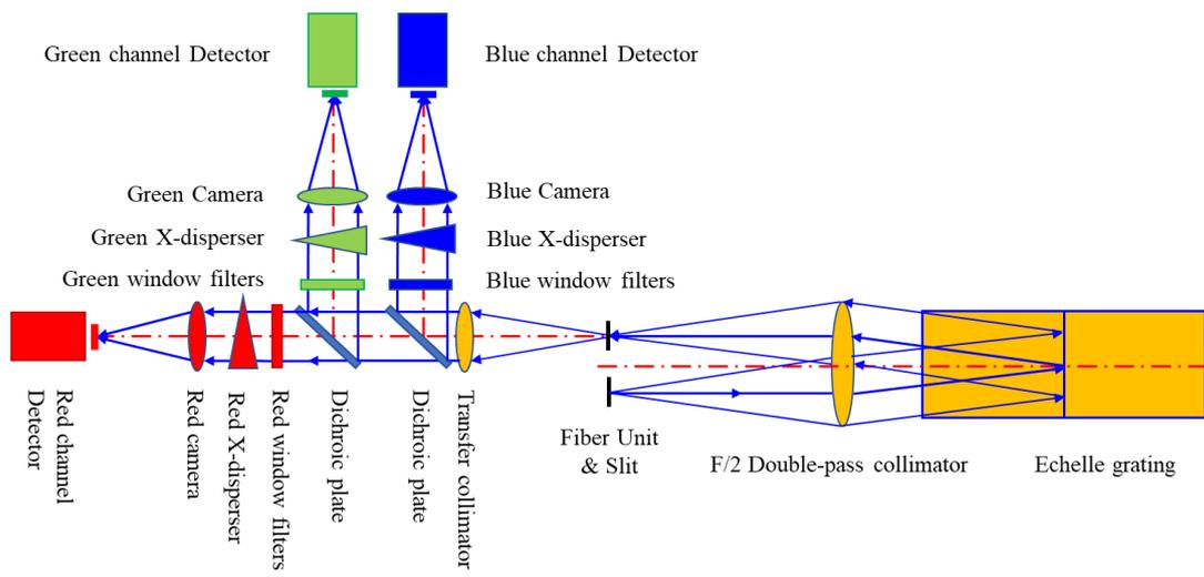
Figure 2. Schematic diagram of a transmissive design based on echelle grating in 2020
