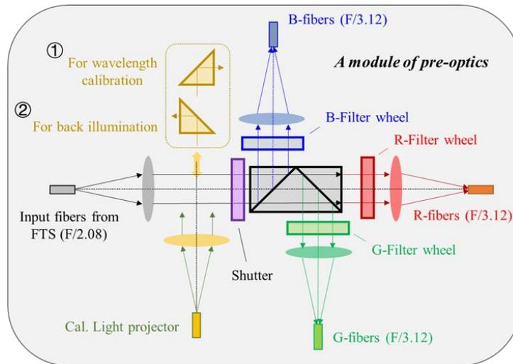
Figure 7. A scheme to inject calibration light from the pre-optics
