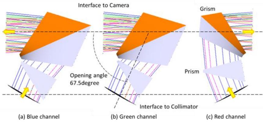
Figure 1. Design of the combination with grisms and prisms in 2018
