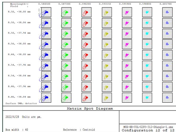
(b) Central wavelength of 593nm at  $m = 38$  in the green channel
