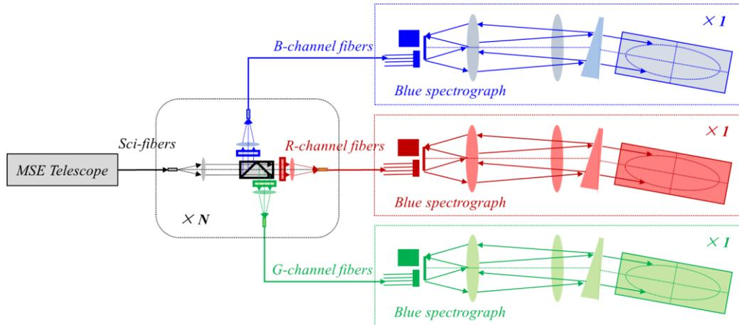
Figure 4. Architecture of single spectrograph units
