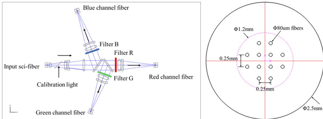
Figure 8. A conceptual design of pre-optics
