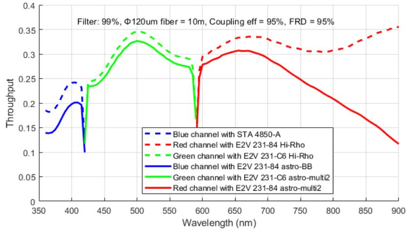
Figure 16. Estimation of instrument throughput
