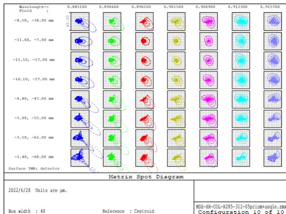
(c) Central wavelength of 900nm at  $m = 25$  in the red channel
