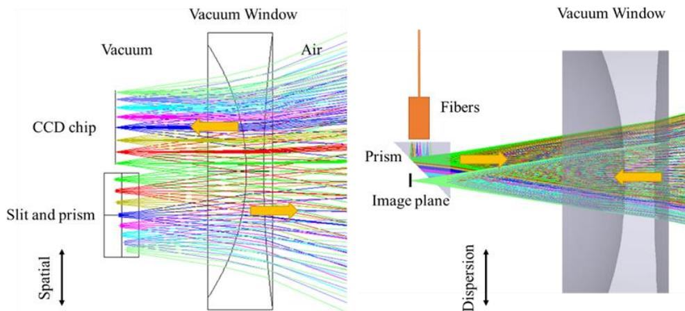
Figure 12. Optical layout of slit and image plane
